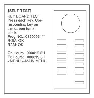
Figure 4-1 Self test screen
